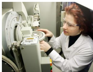
Setting up an X-ray diffraction experiment in the Division of Food Sciences, University of Nottingham, UK
